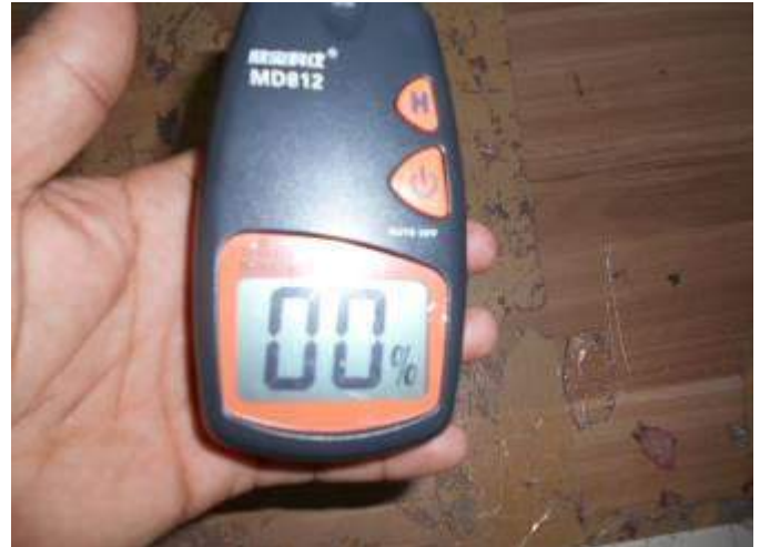
MOISTURE METER ON NUTRAL MODE
